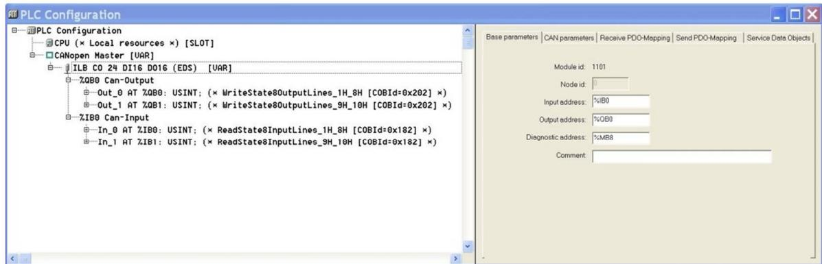
The slave module of the example has 16 outputs and 16 digital inputs associated respectively to addresses %QB0-1 and %IB0-1.
