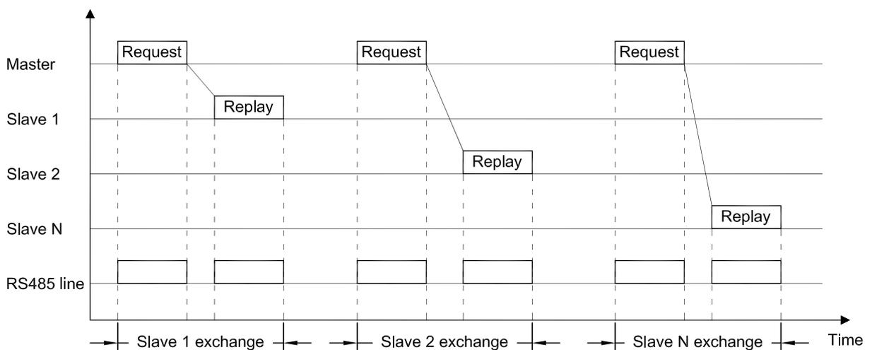
The addressed Slave must replay within the shortest possible time, even in order not to slow down the communication operations with all the others Slave. Additionally, it is important to manage in the Master a predetermined time (Timeout) within which the Slave must replay to avoid blocking the communication in the case of missing or faulty Slave.
