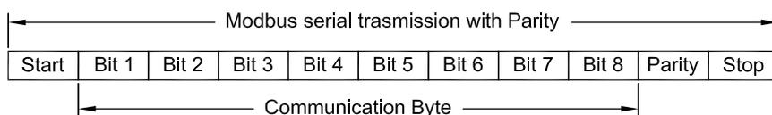
The start bit always applies one 0 level and constitutes a synchronization reference to initialize the reception of all character bits. After the start bit, the 8 bits of the byte are sent starting with
