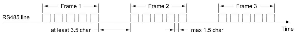
Each frame must necessarily have all its bytes close to each other with a maximum time between the end of a byte transmission and the start of the next, equal to 1.5 times the duration of the character itself.
