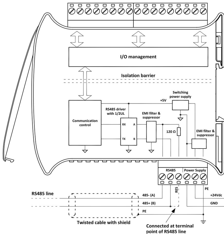
The A and B signals are also indicated as 485- and 485+ by highlighting the polarity of the line in the active driving state of the bit=0, as opposed to the inactive state of the transmission. Note that inactive state, for the presence of the default polarization resistors, assumes the same polarity associated with the transmission of bit=1.
