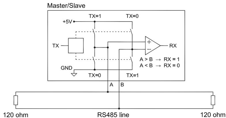
Normally, in the absence of transmission by the device, all four switches of the transmission block are OFF and therefore both RS485 line conductors are not connected to any electrical potential. However, it is preferable not to leave the line floating and therefore a default potential is always applied, positive to A and negative to B. This polarization is obtained by connecting two resistors, one between the power supply + 5V and the signal A and another between signal B and GND reference.
