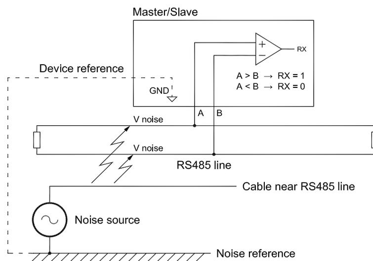
The receivers of each device, which perform a voltage difference evaluation between the A and B wires, will then be able to eliminate this disturbance component because of the same sign and entity on both wires. That is why it is important that any disturbance interferes in the same way with both conductors of the line.
