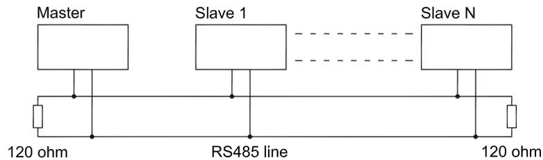
The two-wire connection is as economical as possible but at the same time it offers excellent performance in terms of communication speed and immunity to any electromagnetic disturbance signals. This is thanks to the particular technique of using the electrical signals applied to the pair of wires that will be described below.
